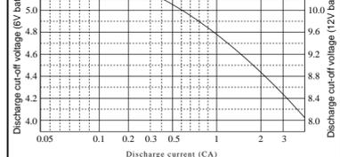
reduction in the number of times of repeatable discharge. When discharging the battery beyond said range, please consult FULLRIVER in advance. (Note) With some types of SLA batteries which have a built-in thermostat, the thermostat may automatically cut off the circuit when discharge current exceeds 4 A at the ambient temperature of 104°F (40°C); therefore, the maximum discharge current value should be the smaller one of either 4 A or 2 CA.
