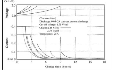
In order to fully utilize the characteristics of SLA batteries, constant-voltage charging is recommended.
